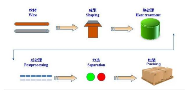
7. Manufacture plant of Silver tungsten electrical contact
